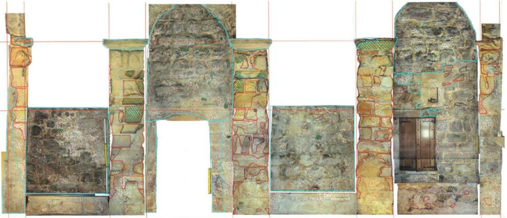
*Fig 2. The condition of the stones recording by Hirst Conservation.*
